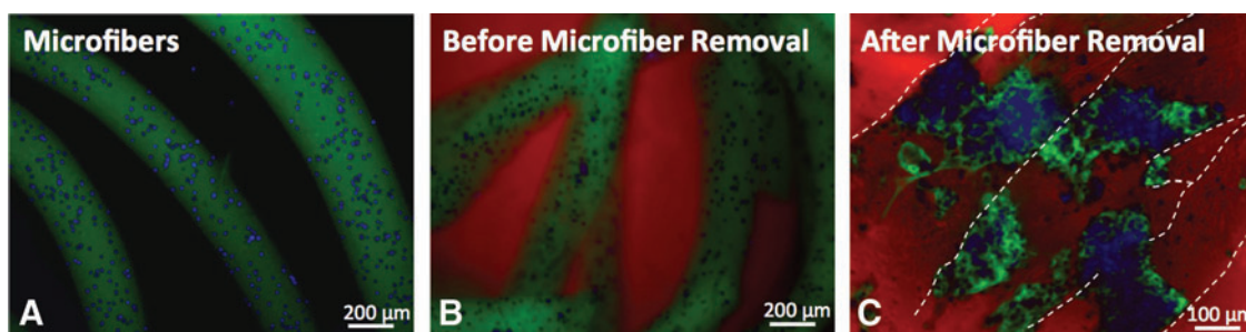
FIG. 4. Fluorescence images of cells in sacrificial microfibers encapsulated within bulk hydrogels. (A) Human embryonic kidney (HEK) cells (Hoechst nuclear stain) encapsulated within fluorescein-labeled alginate microfibers. (B) Cell-containing alginate microfibers encapsulated within rhodamine-labeled bulk hydrogels. (C) After 6 days in culture, HEK cells adhered and spread within the voids left by the degraded microfibers. Cells were stained with FITC-conjugated anti- \alpha -tubulin and Hoechst nuclear stain. Color images available online at www.liebertpub.com/tec
